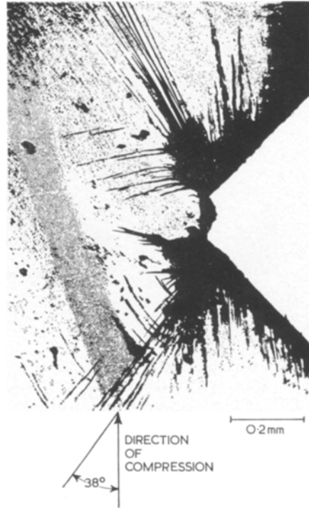
Figure 12 Two deformation band packets radiating out of a notch in a compression specimen of polystyrene (after Argon et al ).
